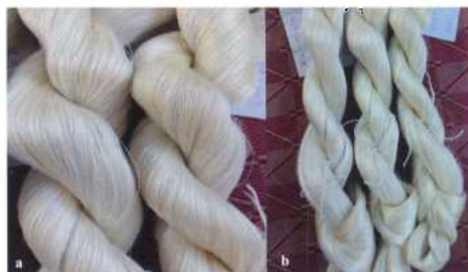
Figure 4: a) Bulky raw silk yarn reeled by cocoon entanglement method b) Multiend machine-reeled raw silk yarn, using equal number of cocoons.
