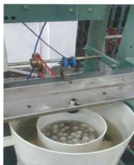
Figure 3: Reeling trials for the production of bulky yarn by cocoon entanglement method
