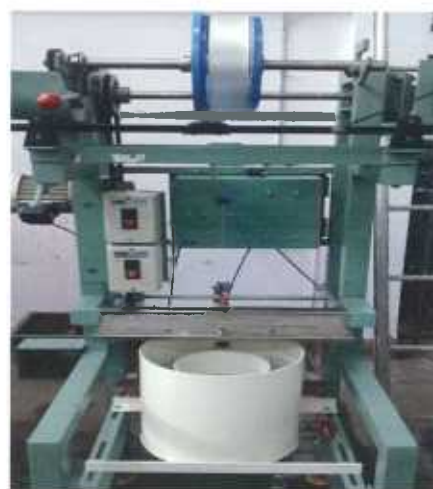
Figure 2: The concept machine developed at CSTRI for the production of bulky yarn by cocoon entanglement method
